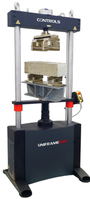
Fiber Reinforced Concrete (FRC) Testing
